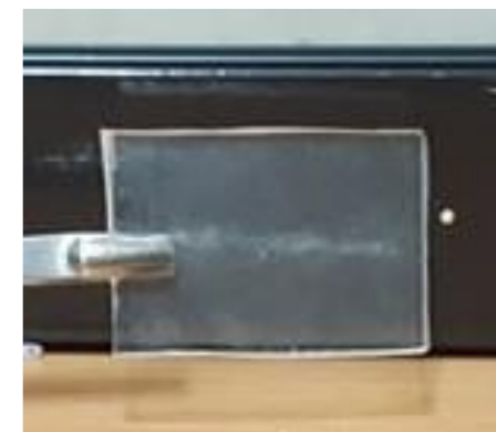
PDMS sample after sterilization in boiled water
