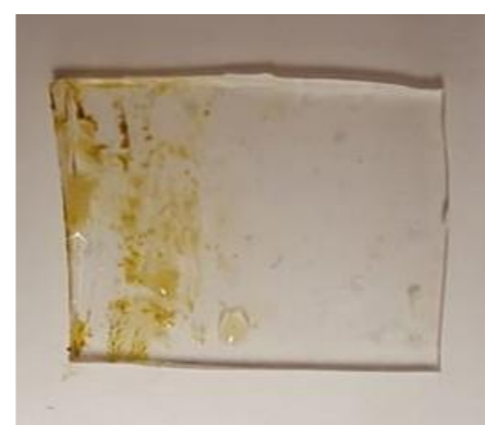
PDMS sample contaminated by microalgae
